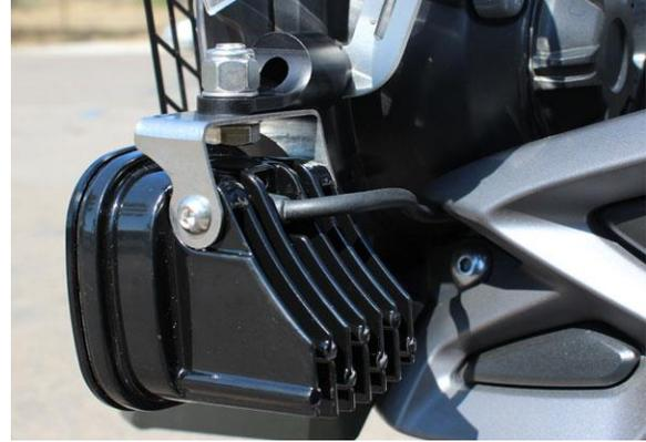
**Step 2:** Now that the mounting bolts have been installed and tightened you can begin mounting your Squadrons or S2 with a 3/8" socket and open-end wrench.
