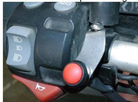
**Step 6.** Locate the black and yellow wires coming off the relay and the red push button switch with two
